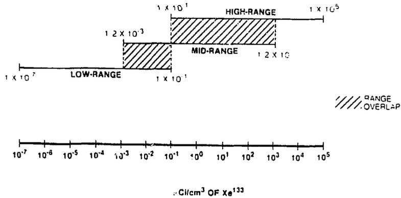
Figure 9. Ranges of General Atomics wide-range gas monitor.
