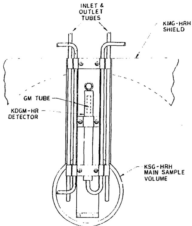
Figure 10. KMG-HRH-Enhanced high-range geometry.
